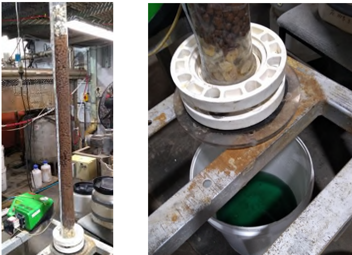
Figure 2: Left photo demonstrates the leach column and the right photo is the pregnant leach solution
