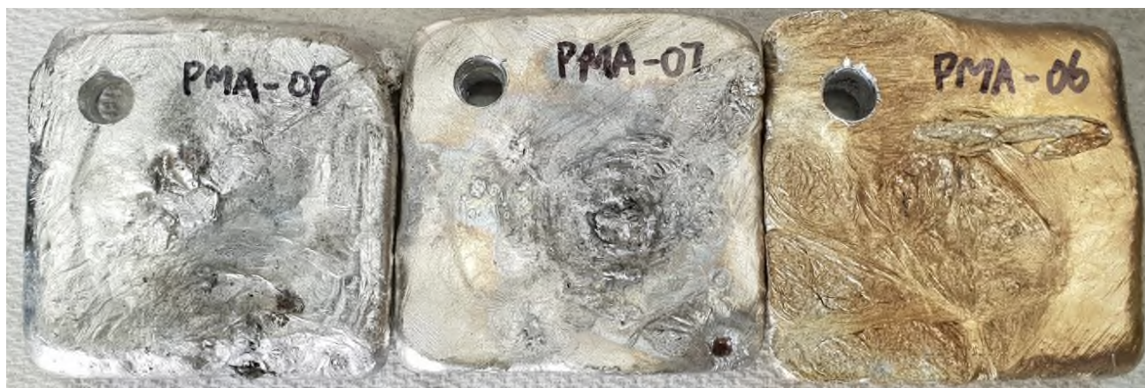
Figure 1 - Master alloys produced from 3 different scandium chemicals from intermediate stages within the PSP scandium recovery flowsheet.
