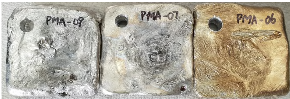
Figure 1 - Master alloys produced from 3 different scandium chemicals from intermediate stages within the PSP scandium recovery flowsheet.
