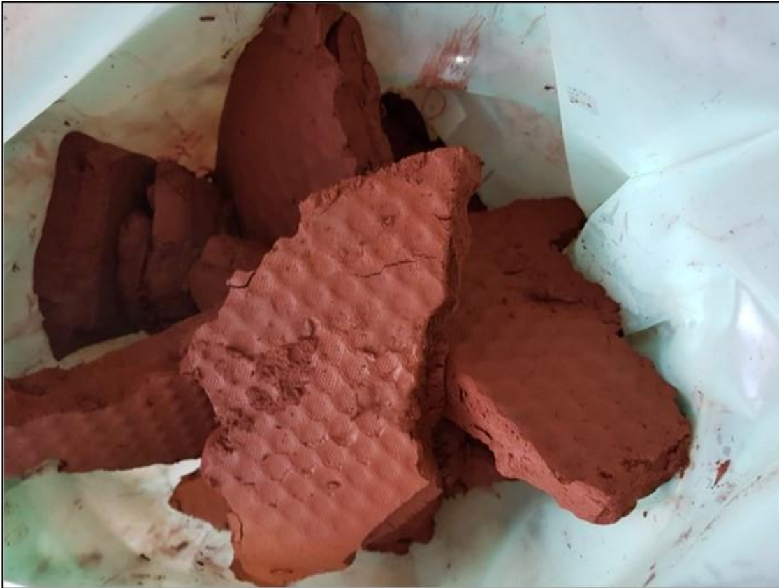
Figure 5 Tailings filter cake produced during pilot plant trial
