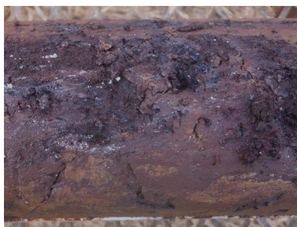
Manganese rich laterite with high Co indicated by hand held XRF
