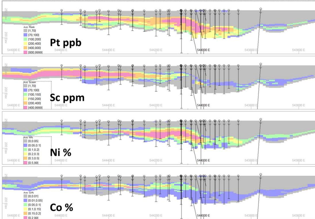
Figure 4. Owendale section 6382815mN - block model grade estimates
