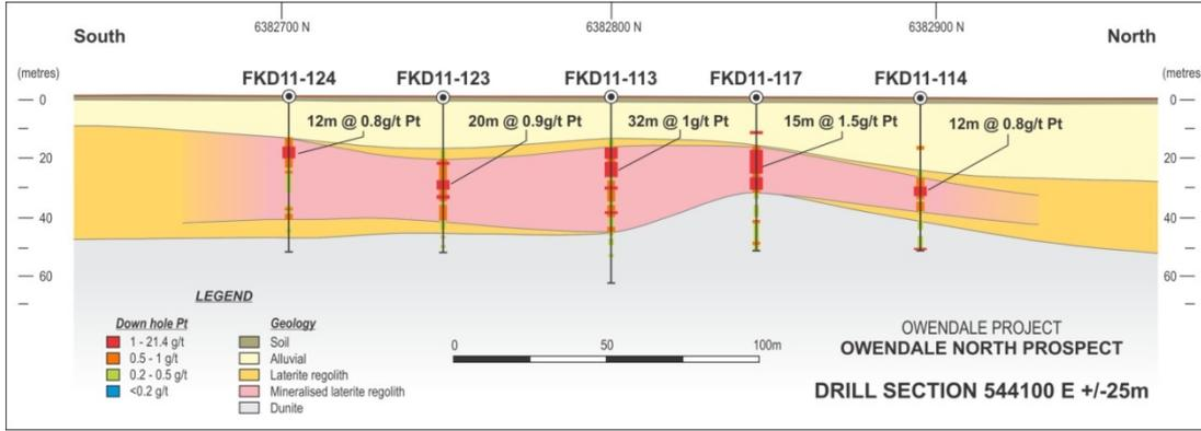
Figure 2. Owendale North - Cross section 544100E
